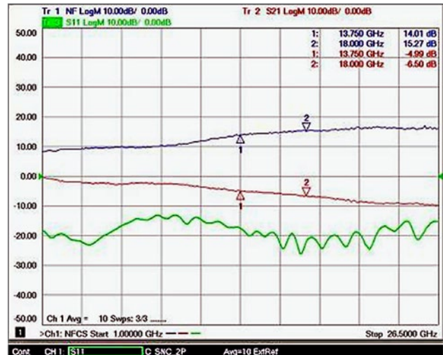
Figure 6. Performance of the same 1.5-km optical link when using the M9405A preamplifier.
