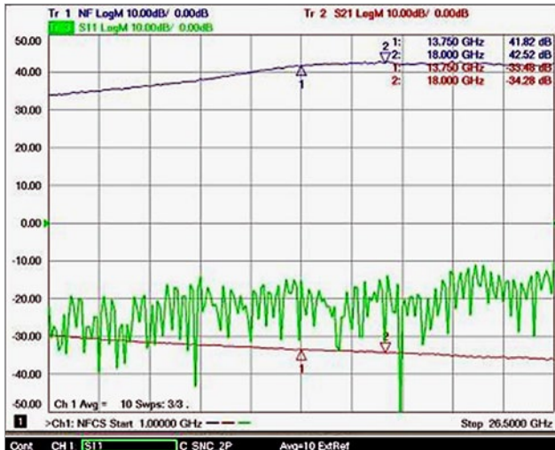
Figure 5. Performance of a 1.5-km optical link without preamplification.
